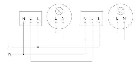
Connection using two-circuit switch for manual and automatic operation
