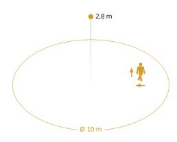
Possible mounting height: 2,00 m - 4,00 m Orange: radial and tangential
